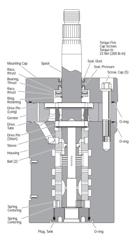
1 Install o-ring (82,6 [3.25] OD) on tank plug.
